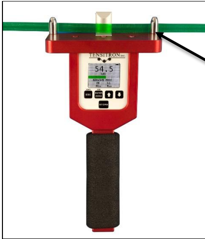
Figure 5: Instrument ready to engage onto strapping.
