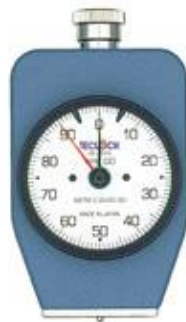
GS-750G Type B Durometer Medium-hard rubber
