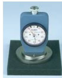
GS-744G Type FO Durometer Soft styrene foam
