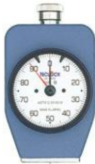
GS-750G Type B Durometer Medium-hard rubber
