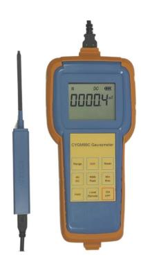
The Gaussmeter CYGM99C works according to Hall Effect measuring principle. It is a microcontroller-controlled instrument and can be used to measure DC/AC magnetic field strength of permanent magnet materials, motors, speakers, magnetic sensors/ transducers, other machines and instruments etc. with high resolution. It is powered with a rechargeable LiPo Battery (+3.7V) or via USB cable (+5VDC).
