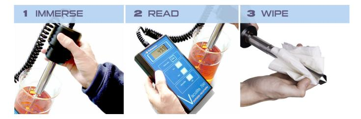
The solid stainless-steel sensor is simply immersed into the fluid to obtain an immediate viscosity measurement. There is no limit on vessel size or fluid volume, so long as most of the probe is covered. Simply wipe clean after use.
