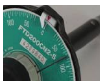
Memory pointer captures peak torque
