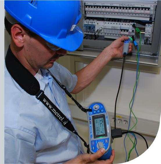
MI 3100 s EurotestEASI is a fast, accurate and easy to use multifunctional measuring instrument which performs a basic set of installation safety tests according to IEC/EN 61557. Besides, the MI 3100 s EurotestEASI enables on-line voltage monitoring, phase sequence testing and earth resistance measurement. EurotestEASI is equipped with integrated characteristics of fuses and RCDs for PASS / FAIL evaluation of test results.
