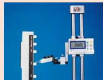
Checking accuracy of height gage
