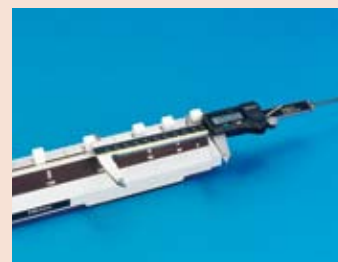
Checking accuracy of caliper (inside measurement)
