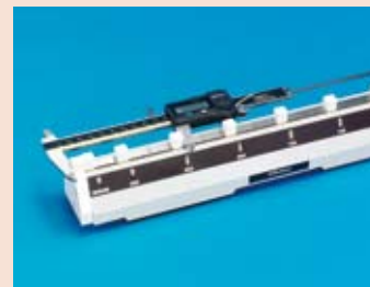
Checking accuracy of caliper (outside measurement)
